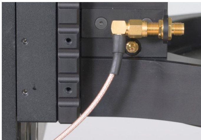
Figure 33: Connection of the SMA plug of the measuring cable to the SMA connector on the rotary unit
