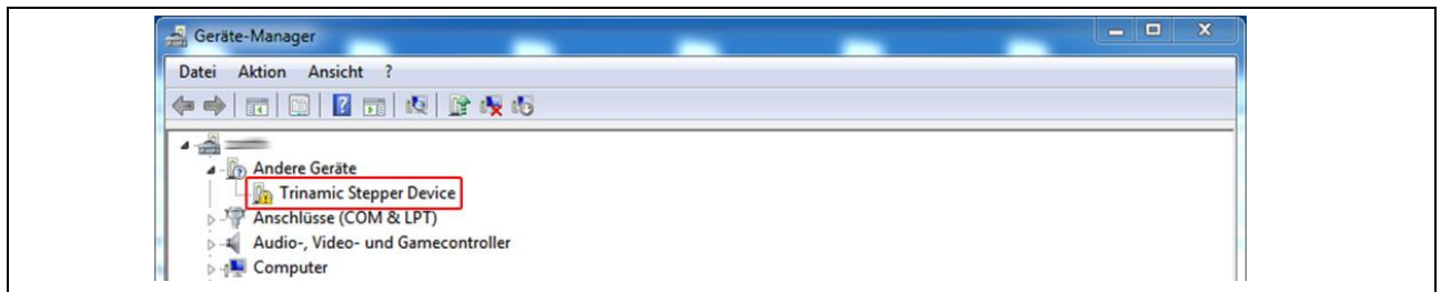
Figure 56: Device manager with the "Trinamic Stepper Device" entry and a warning sign
