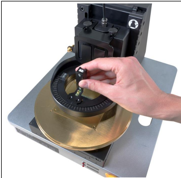
Figure 45: Placing the SH 01 on the rotary ring
